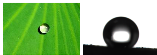
Fig. 2. Lotus Effect and Ashine Fluorinated Graphene Nanoplatelets Contact Angle Analysis
